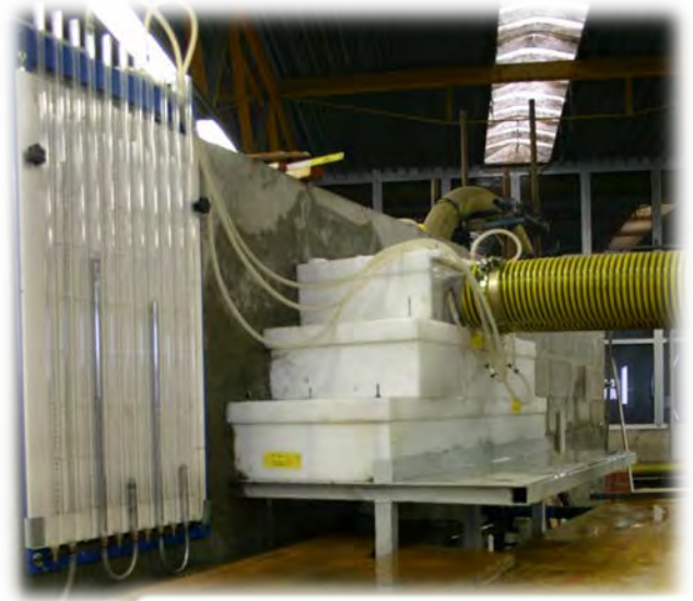
Fig. 7 – Physical model of the intake work (laboratory)
