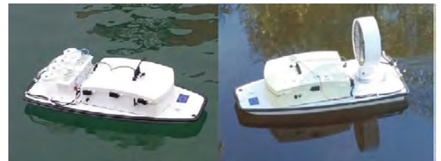
INTCATCH water drones powered by a propeller (on the left) or a fan (on the right).
